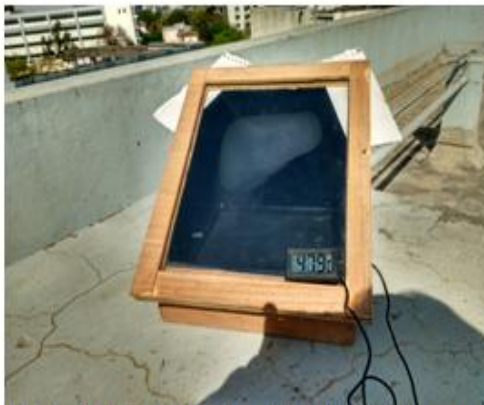
Fig.2 : Fabricated solar still with Thermocouple
